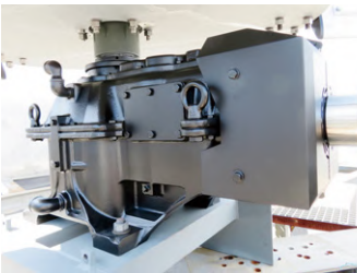
Bevel Gear Drive (B.G) Fan is rotated by transmitting the rotation of electric motor to gear reducer.
